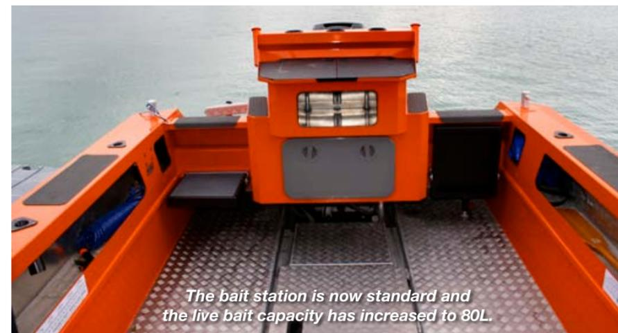
The bait station is now standard and the live bait capacity has increased to 80L.
