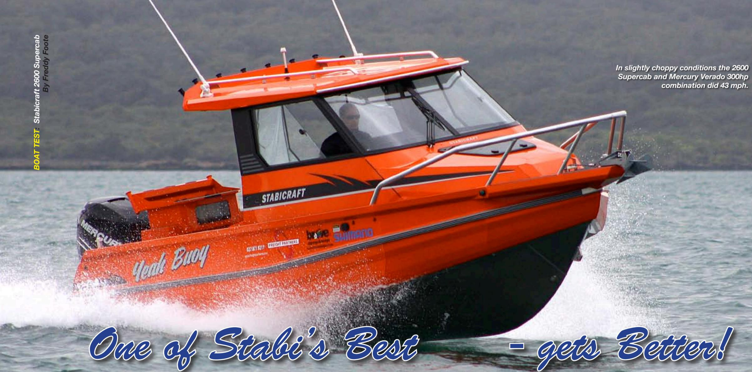
In slightly choppy conditions the 2600 Supercab and Mercury Verado 300hp combination did 43 mph.
